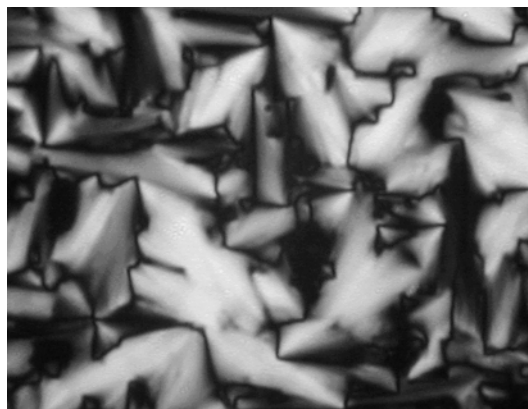
Fig. 2 The fan texture of the mesophase of [C 14 H 29 -imH][NO 3 ] at 70 °C.
